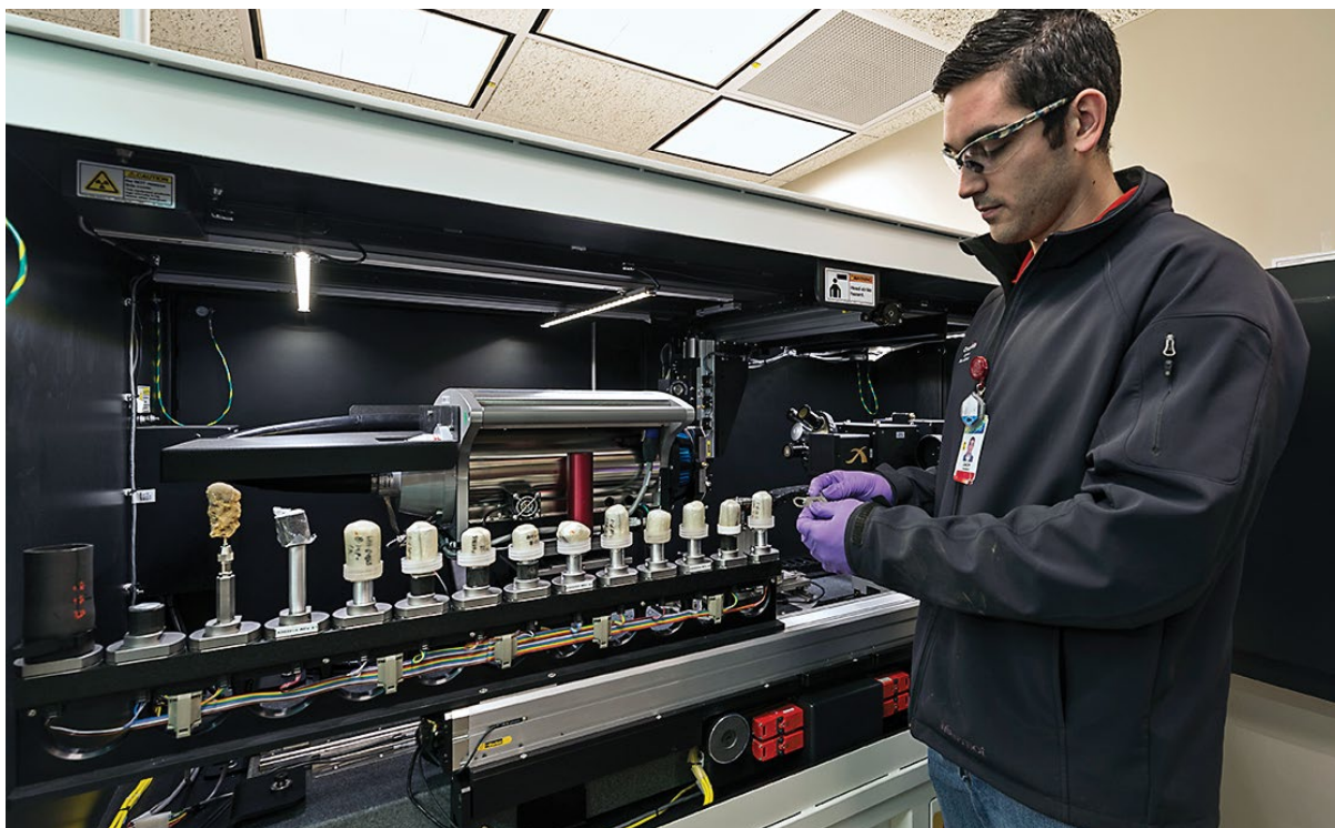
Unconventional Reservoirs Technician Zach Cramer loads core samples into the micro-CT X-ray instrument. The device generates high resolution images of micro-fractures, a unique characteristic of unconventional reservoir rocks.
